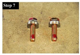
After the rotor is installed and clamped in place, it is time to install the caliper saddle which should have the caliper removed from it. Prep the two caliper saddle to knuckle bolts by putting a the washer and spacer on. That is for the late model unit bearings. The early model will only get the washer under the head of the bolt and the spacer will go between the caliper saddle and the hole in the knuckle to move the saddle outboard for the taller unit bearing.
