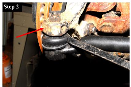
To remove either the draglink or tie rod from the steering knuckle, place a pry-bar over the top of the bar as shown and wedge it under the steering arm. Apply downward pressure and strike the end of the steering arm with a medium ball peen hammer in the direction the arrow indicates.
