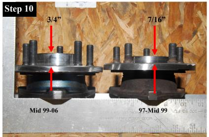
The TJ came equipped with two different unitbearings depending on when it was made. The later mid 99-06 is shown on the left and the early 97-99 is on the right.
