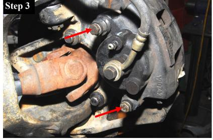
Remove the two caliper mounting bolts and hang the caliper back out of the way. Leave the flex hose connected until it's time to install the new calipers.
