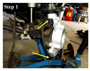
Install the knuckle onto the ball joint pins. Tighten the castellated nuts in accordance with factory recommended specifications. Once they are installed, insert a new cotter pin into each hole and bend the ends over.
