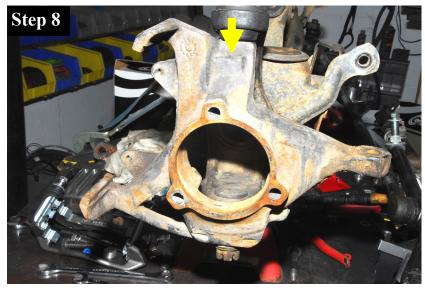
Thread the lower nut back on a couple of turns to catch the knuckle after it's popped loose.
