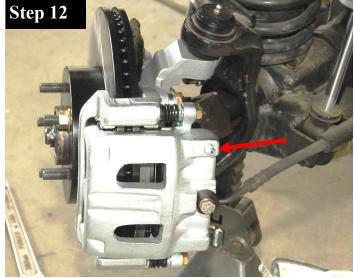
The caliper gets installed next. Make certain that the bleeder screw indicated by the red arrow is above the flex hose. Install the flex hose with two crush washers and the banjo bolt.
