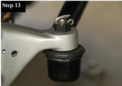
After the brake lines are installed, it's time to put the steering back together. Push the tie rod ends back into the tapered holes in both steering knuckles, tighten down the castellated nuts to factory torque specifications, insert and bend over the cotter pins.
