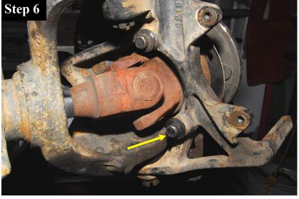
This shows the third of the three flange head bolts that need to be removed. After they are removed, pull the axle shafts and unit-bearing as an assembly and set aside for the time being. Take care to keep the splined area and the seal surfaces clean and undamaged.
