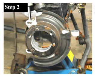
Insert the 3 factory unit bearing bolts into the holes in the knuckle and hang the dust shield on them.
