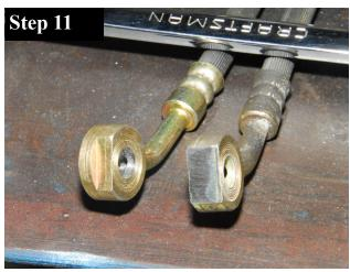
If you are re-using the stock brake lines, the banjo fitting will need to be modified by grinding the shoulder off shown on the left until it is flush like the one on the right.
