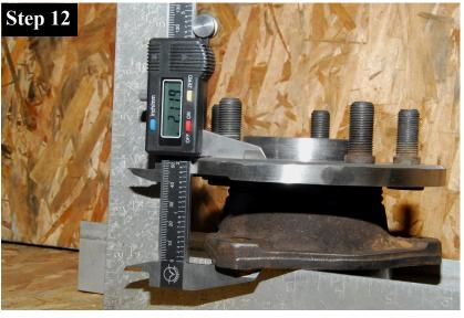
The early unit-bearing is shown and the dimension is 2.119" or slightly under 2 1/8".
