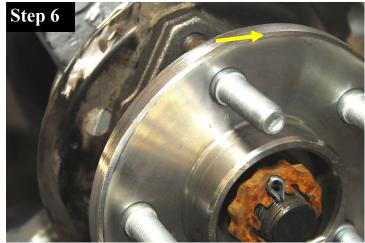
The arrow indicates the new 45° chamfer that has been put back on after the grinding to fit is finished. This is important so that the edge of the flange does **not** contact the small radius where the rotor hat flat face meets the side wall of the hat. If there is contact, the rotor will wobble and dramatically decrease brake performance.
