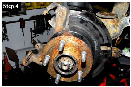
Remove rotor to access unit bearing as shown.
