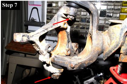
Remove cotter pins and castellated nuts from both the upper and lower ball-joints.
