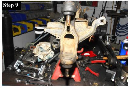
At this point you should have your inner C looking like this. This is a good time to inspect the upper and lower ball-joints and replace them if needed.
