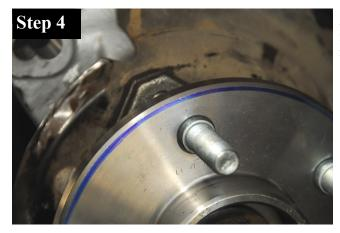
A closer view is shown. The reference line is to show the minimal amount of material that needs to be removed to fit the new rotor hat over the flange. A grinder with a coarse grit sanding flap disc works well for removal.
