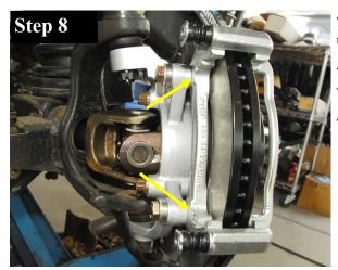
This shows the correct orientation of the spacers for the late model unit bearings with the spacer between the washer and knuckle.
