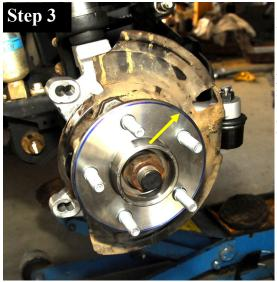
Install the unit bearing and axle assembly into the knuckle, thread the unit bearing bolts into the holes and tighten them to 75 ft. lbs.
